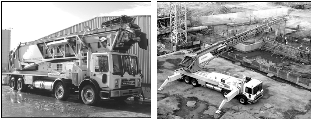
Figure 9. Putzmeister Telebelt used for placing RCC at elevated and restricted access areas
